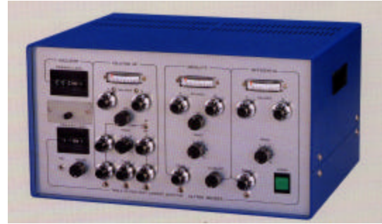
The ULTRAY ND-382 multifrequency Eddy Current instrument
