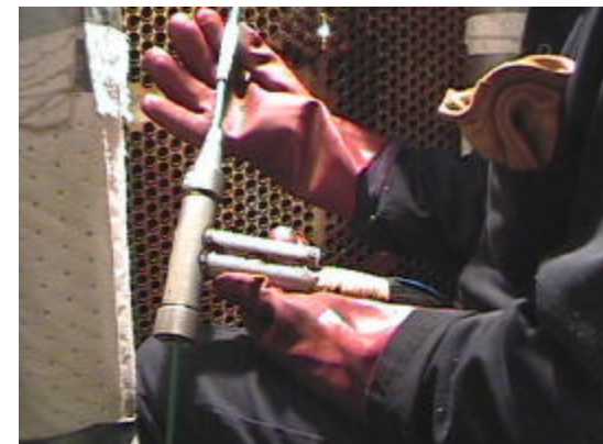
The insertion device for the automated probe pusher/puller
