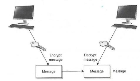
Symmetric cryptography is 1,000 times faster than Asymmetric cryptography
