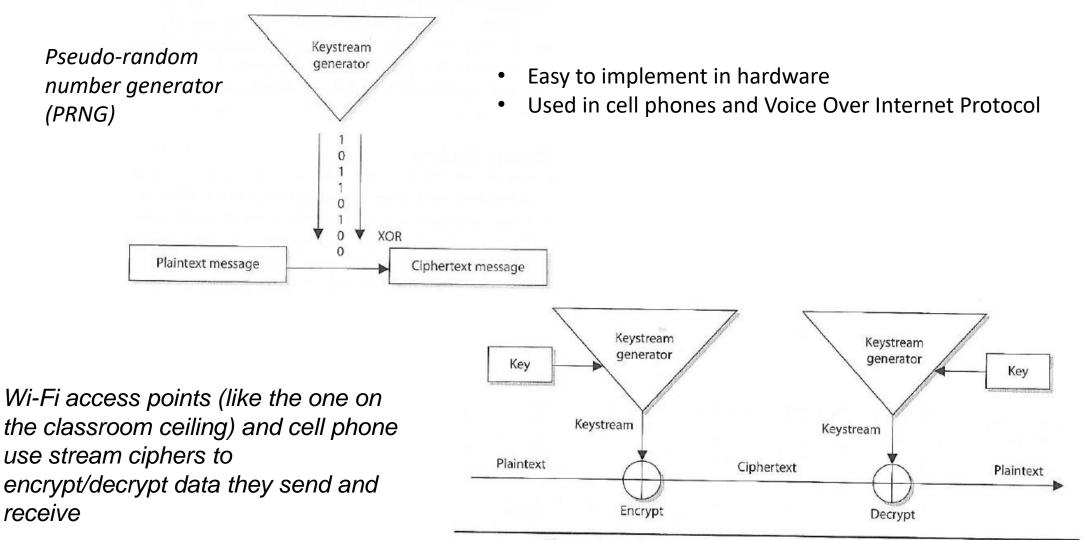
The sender and receiver must have the same key to generate the same keystream.
